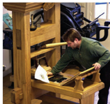
Source 3.58 A reproduction of Johannes Gutenberg's printing press. It used movable type, arranged within wooden frames, to print a page of text.
